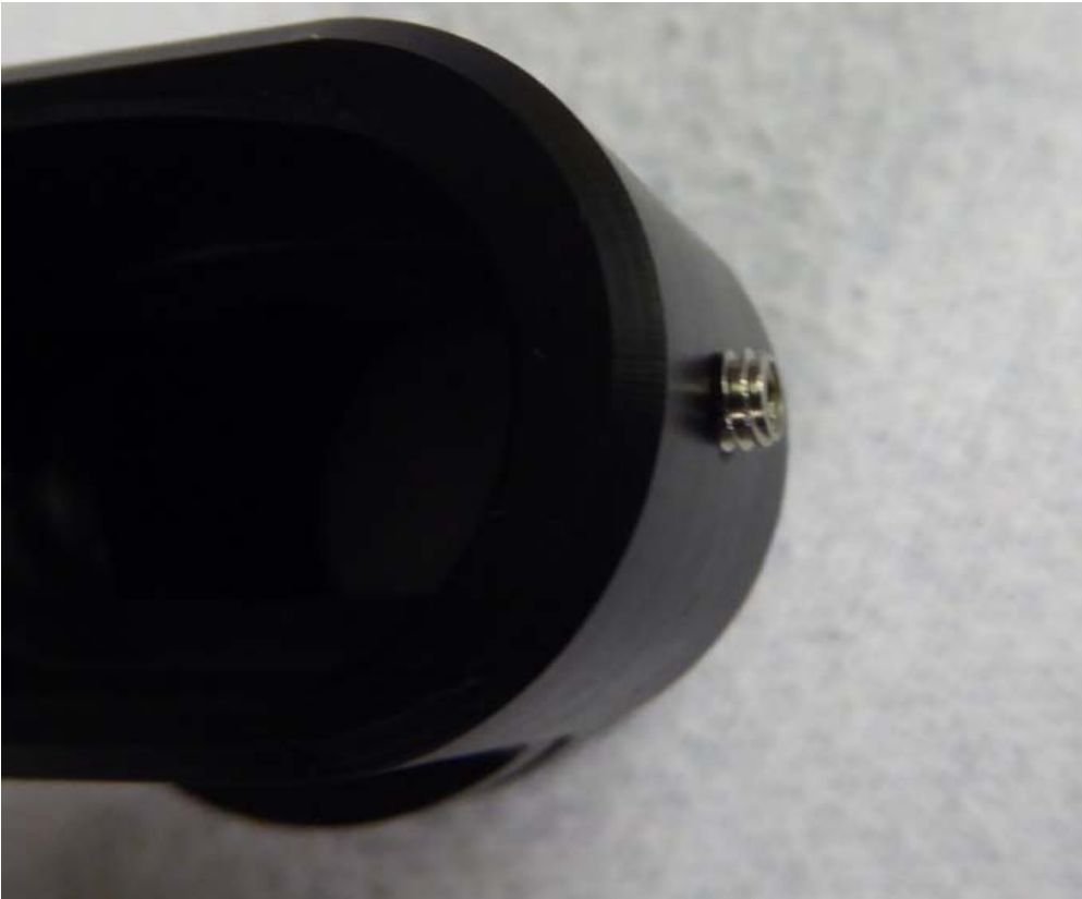
take care the set screws are out, so they are not staying inside!
